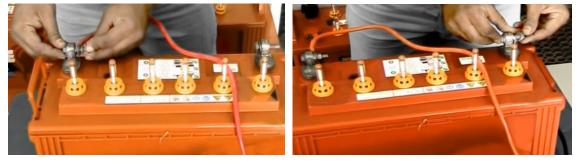
Fig 3.1.9: Connect the battery terminals
