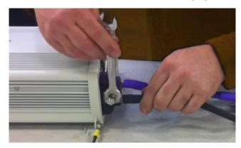
Fig 3.1.10: Attach leads to the inverter
